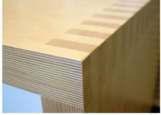
The use of high gloss finishes and paints tends to highlight naturally occurring and manufacturing characteristics of plywood such as beat marks from sanding, knots and open defects in underlay veneers, grain variation and patches, and is therefore not usually recommended. Stain and matt finishes and paints give a high quality aesthetically pleasing surface and are recommended.
